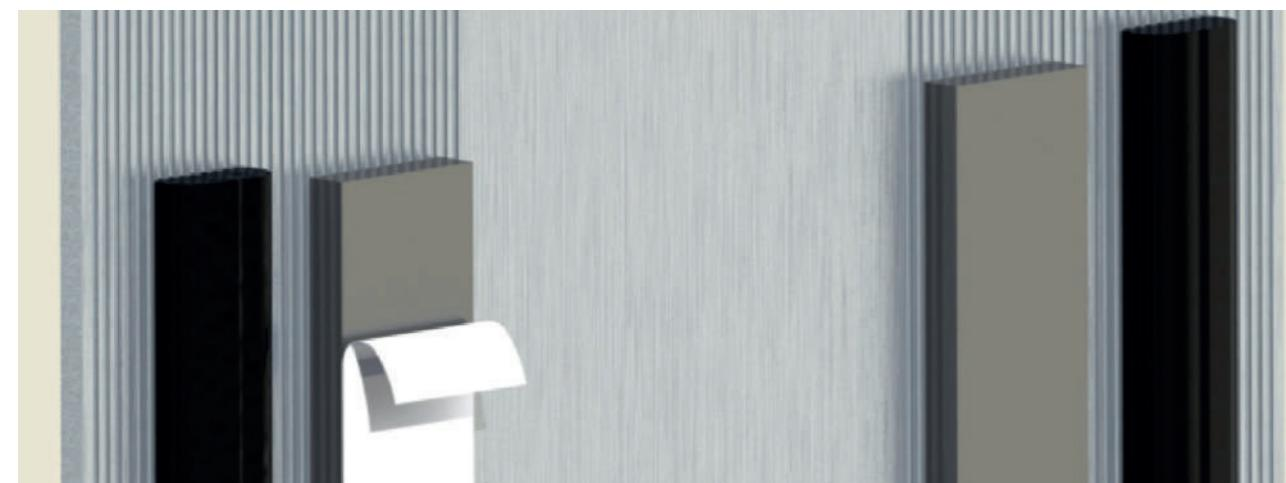
Two beads of elastic adhesive are applied along the vertical T-profile and a single bead on the L-profile, specifically in the grooved area of the profile. The adhesive ensures the correct positioning of the chosen panels, improving the system's responses to gravitational loads, pressure loads and wind suction, absorbing vibrations and thus avoiding possible clapping.
