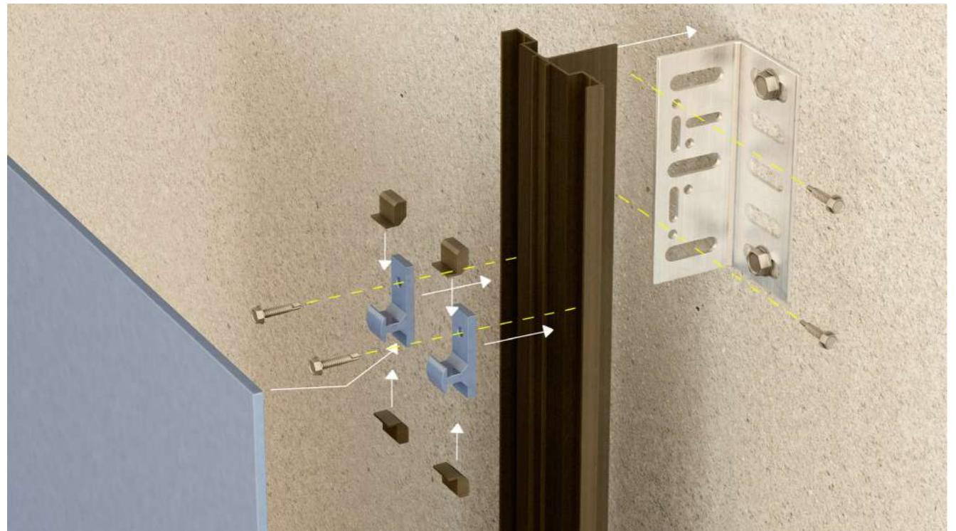
The ARKTECH VST SYSTEM is a self-supporting aluminium and stainless steel metal substructure kit for ventilated facades and designed for Arklam Slim 6 mm cladding. The system is composed of support and retention brackets, vertical profiles and staples on which the cladding rests, all in high quality Aluminium T5 6063.
