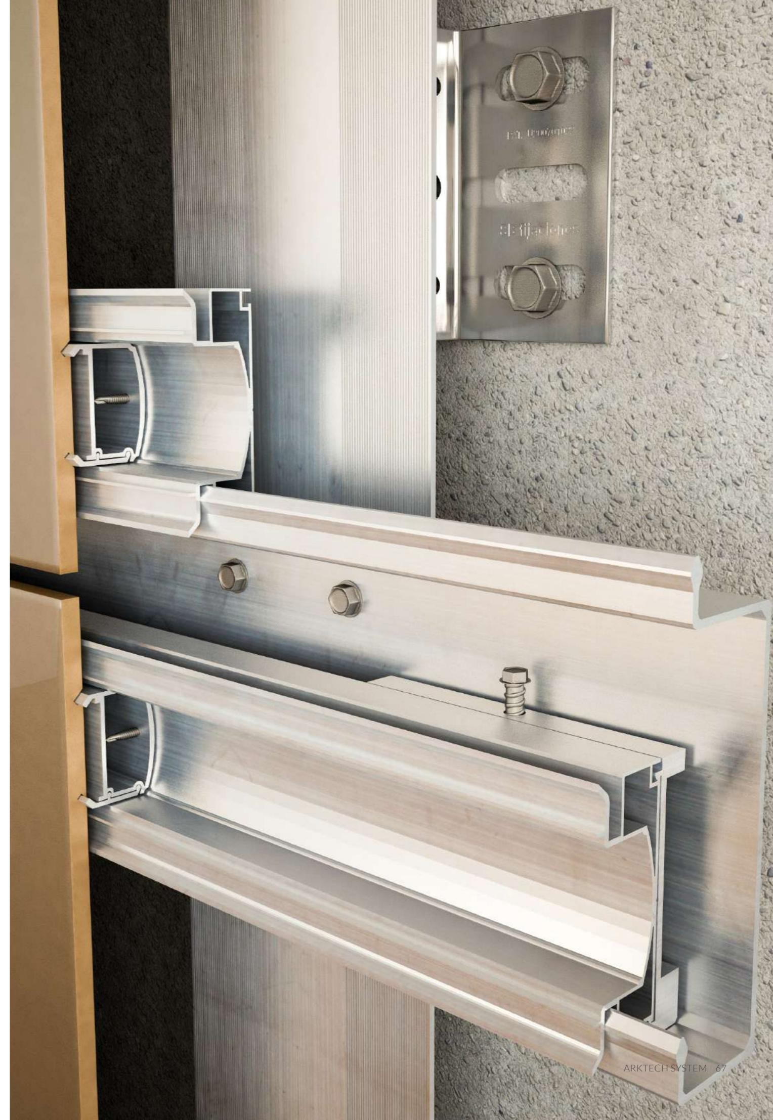
This system consists of sustentation and retention brackets, staples, vertical T-profiles and horizontal profiles with geometry designed exclusively for this purpose.
