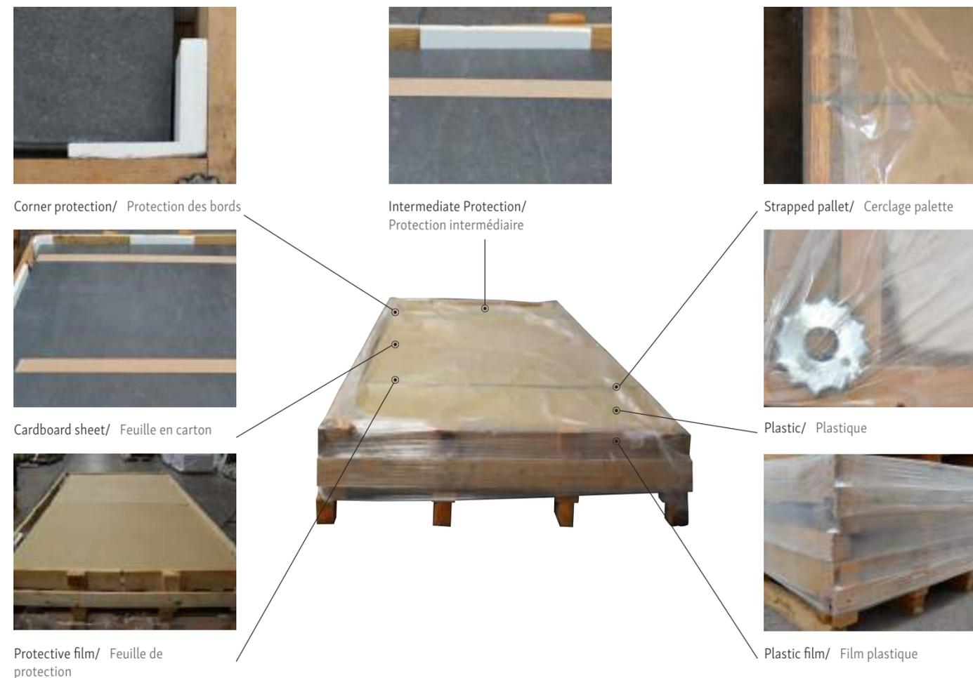
Arklam is supplied in special packing. Arranged in 2860x1620x360 mm / 3180x1120x305 mm wooden crates, suitable with a more secure structural system, through lateral reinforcement arranged to support the loads caused by the Arklam sheets contained within, as well as a longitudinal reinforcement to transmit those loads both at ground level as well as carrying out stacking between the different trays, which also helps to protect the load for collection outside.
