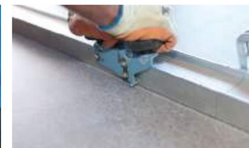
For the execution of a dry cut of the ARKLAM piece, cutting guides with suction cups are used. The guide will be set and its position fixed.
