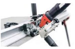
With a special bevelling machine supported on the ARKLAM With a special bevelling machine supported on a guide of adjustable nylon pulleys, offering total precision in the work.
