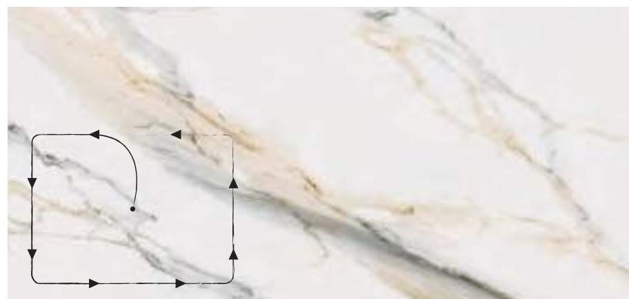
The slab must lean completely on the machine ribs. We always recommend to finish the cut towards the edge of the slab, whenever the machine's software allows it. The first and last 30 cm must be cut at a speed 50% lower than initially recommended. Start in the groove's inner part and move towards the cutting line at a speed of 60% when performing the groove in order to avoid chipping. Use brackets to prevent the pieces from moving.
