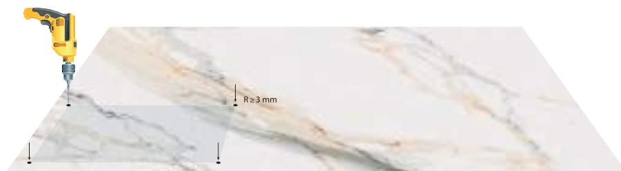
To adjust the angle before cutting a groove, we must first perforate all its corners with a drill bit of  $> 3$  mm. radius.
