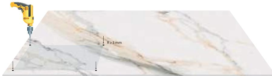
To adjust the angle before cutting a groove, we must first perforate all its corners with a drill bit of  $> 3$  mm. radius.
