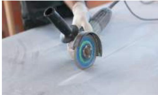
In order to make a dry or cool cut in the ARKLAM piece by means of diamond disk, the use of support guides at all times is recommended.
