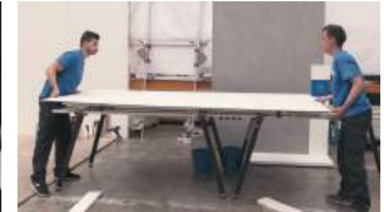
For the cutting, drilling and finishing of the edges of an ARKLAM sheet, a suitable workbench both in terms of rigidity and in planimetry, and which supports the weight of the piece, as well as maintaining the entire surface, should be prepared, to allow cuts to be made at the different points intended.
