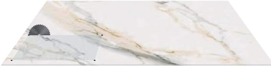
Secondly, we shall unite these punches with straight cuts using the cutting bridge disk at a minimum speed to prevent breakage, since at this precise moment the slab is under a lot of pressure.
