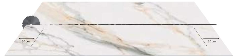
During cutting process, the disk must be refrigerated with plenty of water, and the water jet must aim directly to the cutting point, where the disk is in contact with the slab, since ARKLAM's sintered mass is a dense and hard material. We suggest cutting the first and last 30 cm at a lower speed than recommended (50%) in order to improve the cutting finishing.
