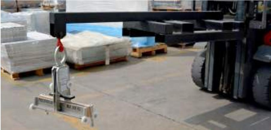
To pick up slabs individually, use always alligator or conventional clamps, with vulcanized rubber at the contact points to avoid the risk of slipping and moving, while complying with the maximum permissible load. The pieces must be removed alternately on each side of the easel to compensate the weight and avoid overturning.
