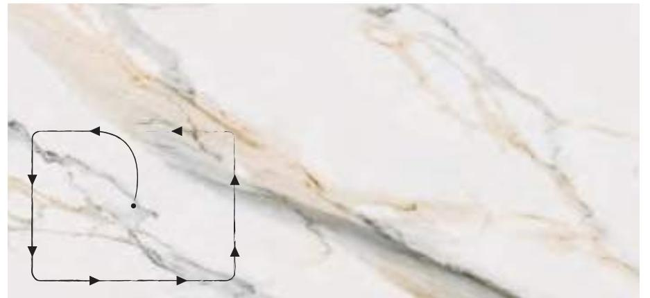
The slab must lean completely on the machine ribs. We always recommend to finish the cut towards the edge of the slab, whenever the machine's software allows it. The first and last 30 cm must be cut at a speed 50% lower than initially recommended. Start in the groove's inner part and move towards the cutting line at a speed of 60% when performing the groove in order to avoid chipping. Use brackets to prevent the pieces from moving.
